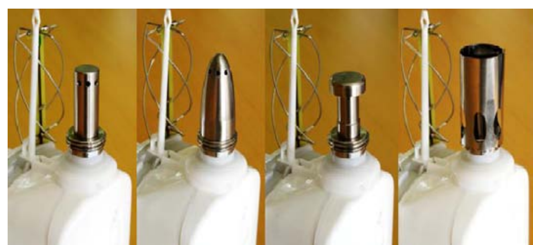
Figure 2. Wind shield types 1...3 and a radiation shield
