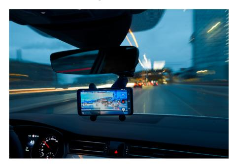
Traditional road pavement condition surveys are mostly performed manually, subjecting the process to human errors and delays, and further draining limited resources. With Vaisala RoadAI, part of our Xweather family of subscription based products, pavement assets can be evaluated thoroughly and objectively for efficient management at a fraction of the price of manual evaluations.
