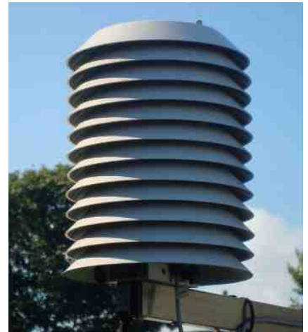
A Vaisala HMP45D relative humidity sensor with Vaisala DTR13 radiation shield installed at a Finnish Meteorological Institute site. Dew point calculations are carried out by the central data collection system.
