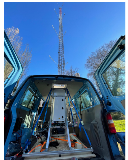
Mobile Ceilometer CL61 being prepared for measurements in front of a 40 m meteorological tower operated by Technische Universität Berlin. © Andreas Christen
